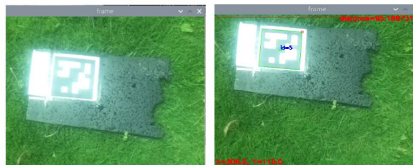
FIGURE 15. Intermittence in the detection of the marker in consecutive frames caused by the influence of direct natural light on the marker
