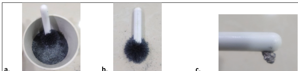
Fig. 6. a, b) Activated catalyst, and c) Residual sludge after Fenton Process magnetic characteristic.
