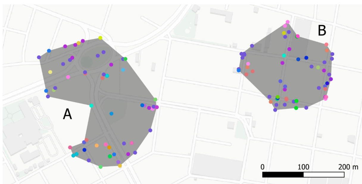
Figure 3. Example of concave hull footprints for two sets of 60 points to estimate land use density and diversity. Colors represent different land use categories. (A) area = 5.6 ha, density = 10.7 pts/ha. (B) area = 2.9 ha, density = 20.5 pts/ha.
