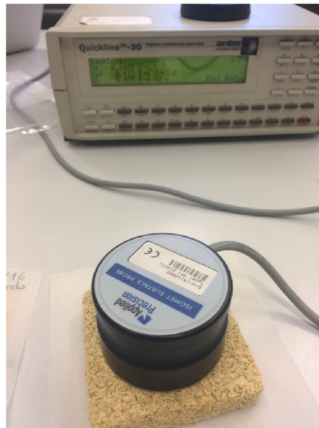
Fig. 5. Quickline-30 Thermal Parameter Analyzer with an Isomet surface probe API 210411.
