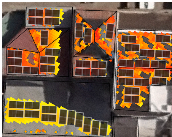
Fig. 10. Manual distribution of PVs on suitable surfaces.
