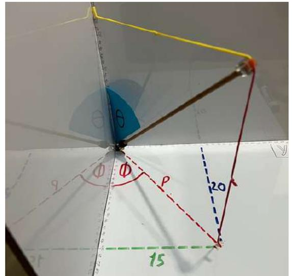
$$r = \sqrt{x^2 + y^2 + z^2} \rightarrow r = \sqrt{20^2 + 15^2 + 23^2} \rightarrow r = \sqrt{1154} \quad (\text{Decimal: } r = 33.97057\dots)$$
