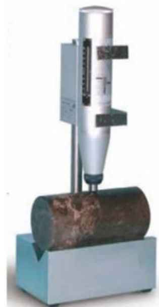
Figura 06: Esquema de martillo de Schmidt Antonio Lozano GEOENGINEERING SERVICES & CONSULTING E.I.R.L
