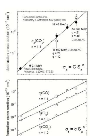
Figure 1: Cross section for destruction of CO<sub>2</sub> (top) and synthesis of CO, CO<sub>3</sub> and O<sub>3</sub> (bottom) as a function of electronic energy loss.
