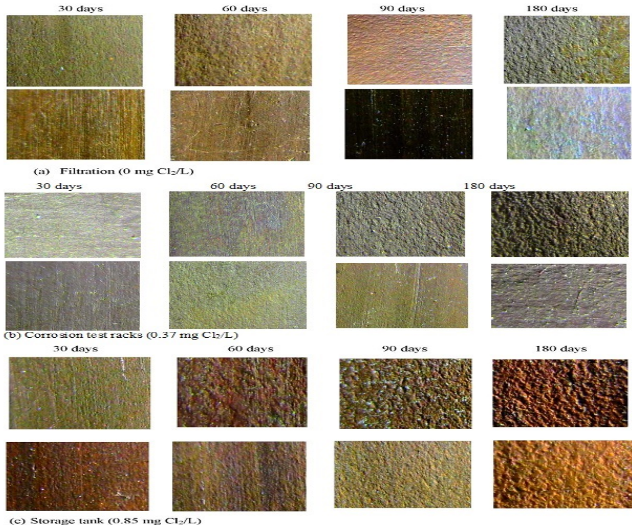
Fig. 9. Image of corrosion of the copper coupons
