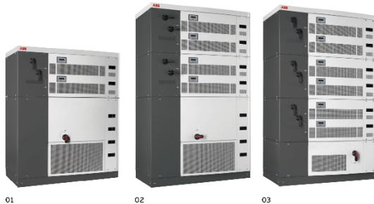
ABB's central inverters are extremely scalable, modular-inverter systems that are based on 55 kW modular blocks. This increases usable power and improves availability. The reduction of performance in any individual module will not impact the energy harvesting capabilities of the other modules.
